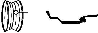
VIEW 1. RIM WITH NO HUMP AND WITH VALVE HOLE ON WEDGE LEDGE SIDE. MOUNT AND DEMOUNT WITH VALVE HOLE DOWN.
