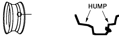
VIEW 2. RIM WITH HUMP ON EACH SIDE AND VALVE HOLE ON NARROW LEDGE SIDE. MOUNT AND DEMOUNT WITH VALVE HOLE UP.
